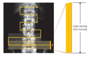
Direct-to-digital detector plus staggered array enhance precision and create high-resolution images.
