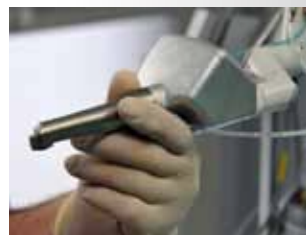
Fig. 2: X-Runner – digitally controlled laser handpiece
